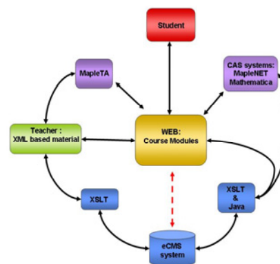
Figure 2: Basic overview of the NS-eCMS functionality, and the location of the previous eCMS system.
