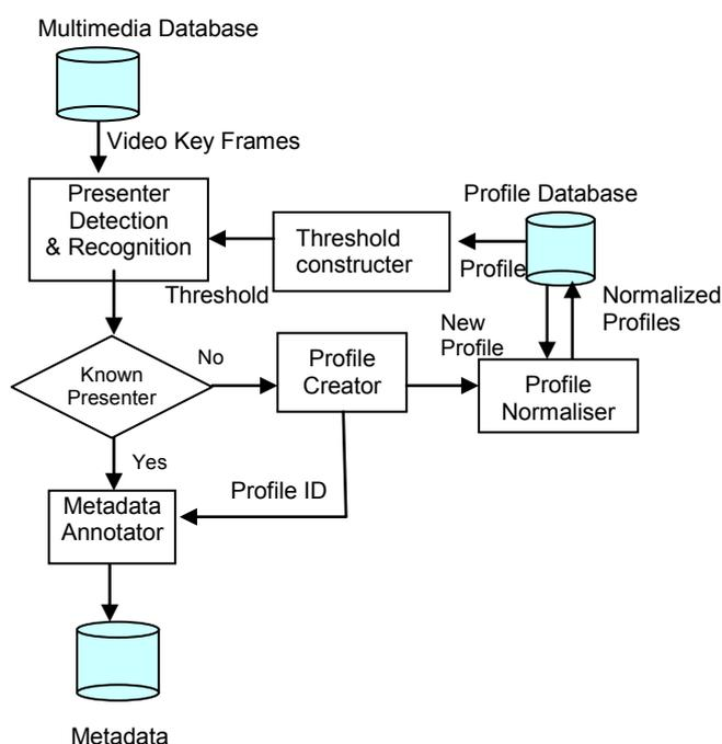
**Figure 2:** Profile construction and recognition process
